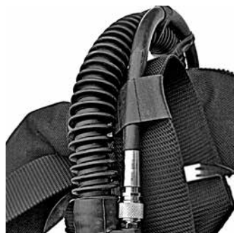
Correct attachment of the inflator hose
